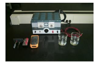
Six stations are prepared as shown in the photo at right. Included are (back row) the power supply, 5 banana plug patch cables, (front row) the coupon holder, 1-ohm resister box, volt meter, tweezers, 150mL electrolyte solution, beaker of water for rinsing.
