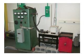
Induction furnace setup: left to right, power supply, service switch (green), crucible box (white), and catch pan (red cart with sand).
