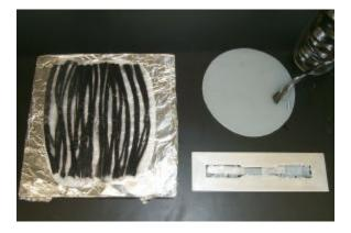
Presses are run at 275 degrees (top platen) and 300 degrees (bottom platen) Fahrenheit. Any material which is squeezed from molds must be scraped off platens before next set of samples is pressed.
