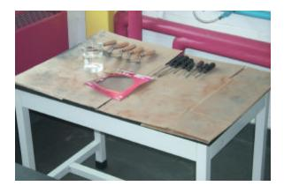
The rust removal station tables are covered with cardboard to protect the tabletops. 12-15 pre-rusted tools and pieces of sand paper are supplied for the first part of the lesson. Coupons are also cleaned here.
