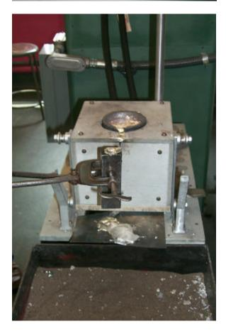
Setup of a bend-bar casting station. Spoon is used to skim liquid metal and remove oxides and other impurities.
