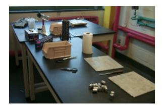
The working/supply area is as shown. Balance, LDPE pellet bin, Cfiber spool, tinfoil rolls, putty "knife", gloves, press platens, adhesion test pieces, paper cutter, and paper towels are available for the students.
