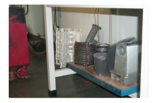
Some of the visual aids used for the introduction to this module. Note the induction furnace water pump on the floor in the background behind the red cart. Extra crucibles and a coil are also visible on the shelf.
