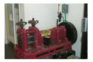
The rolling mill in B-311 must be treated with respect. The power cut-off is on the wall in the background. Samples should be inserted from the near side using tongs provided, then the student should walk around the machine to retrieve the sample, not reach around it!
