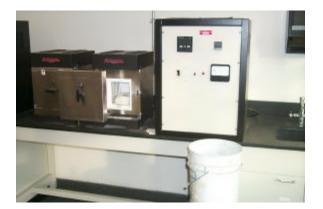
The work-hardened samples are annealed at 300-400degC for 1 hour, then allowed to cool *slowly* on a fire brick, before they are hardness tested again. Ensure students wear goggles and thermal mitts.
