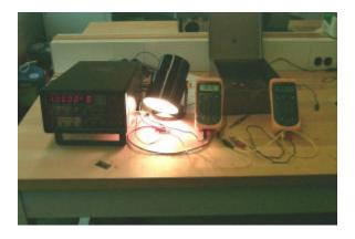
Characterization and data acquisition of data with photonic energy applied to the n-doped side of the solar cell. Similar data is taken with the light not applied. Fourth-quadrant shift (when data is graphed) is used to determine efficiency (the "Fill Factor").
