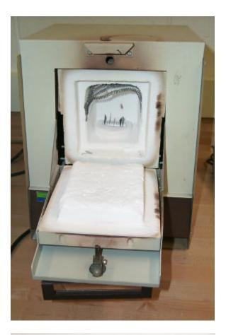
Samples are placed in the annealing furnace after spin coating. They will be annealed for 1 hour at 1000degC, then let cool in the oven overnight. The next day, each group who puts a sample in takes one of the preannealed samples out and continues the module. ~12 samples must be ready (already etched, coated, and annealed) for the first class of each semester.
