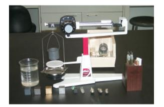
Each of six stations should have a balance, hardness testing kit (with 4 double-pointed scribes), beaker of water, custom weighing basket, and box of 16 material samples (fore and background).
