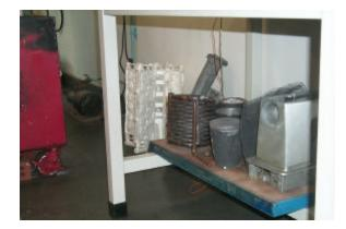
Alloy bar casting station- one of three types of alloy. Note source / recycling container (tan) on right in background. Remind students to resupply the hot pot for the next group's pour while they are waiting for the die to cool so they may move to the next station.
