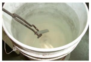
The work-hardened samples are annealed at ~900degC for 1 hour, then quenched, before they are hardness tested again. Ensure students wear goggles and thermal mitts.
