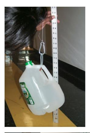
Students are measuring the elongation of fishing line at their respective stations. There are 2-3 types / thickness of line. The known load is 1 gallon of water (~8lbs). Students must be reminded to take readings quickly and provide ample time between readings for relaxation and recovery (1-2 min).
