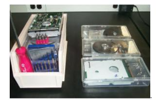
Layout of B-312 setup for reverse design of hard drive module- six stations. Students are guided through the disassembly and evaluation process, referencing all the knowledge they have accrued through the semester.
