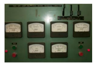
Control panel of the RF furnace generator. Only the power button (out of picture), field and load on/off buttons, and the power level dial maybe adjusted. All other settings must not be changed except by qualified personnel.
