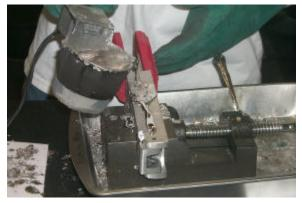
Casting of an Sn-Bi alloy bend bar for alloy effect and property characterization.
